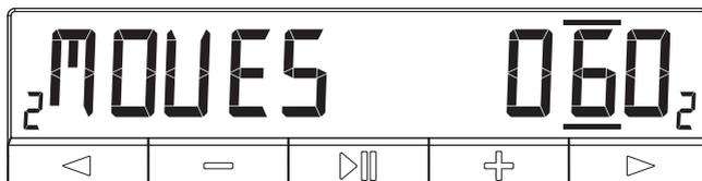
Figure 7. Move counter selection in manual mode
